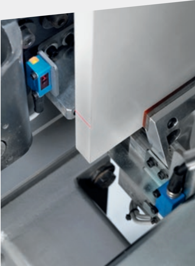
The laser scanner system that detects the start and the end of the panel enables the machine to compensate dimensional errors, correcting the panel's X dimensions.
